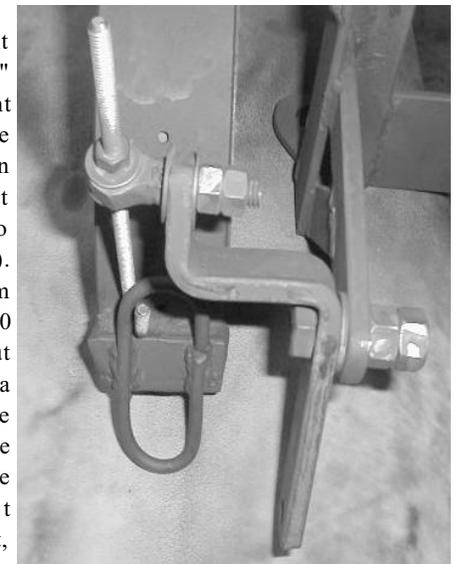
**Fig.7:Control arm (from side)**
