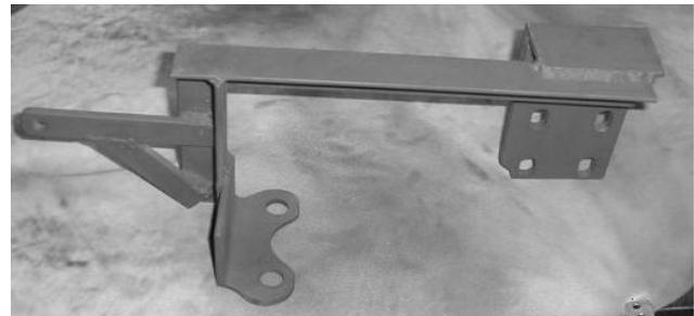
**Fig.5: Mounting arm (from behind & above)**
